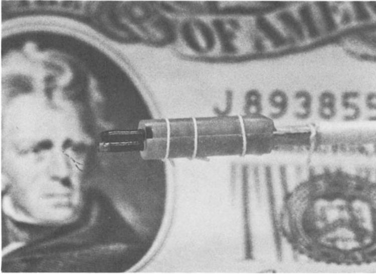
Fig. 2. Pair of detection coils prior to final balancing. The length of the last turn was adjusted (the loose lead is shown) to match the electrical characteristics of the coils. The top, black coil is epoxy filled with oriented superconductor particles.
