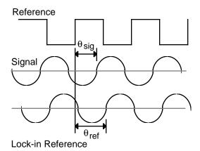
The SR830 amplifies the signal and then multiplies it by the lock-in reference using a phase-sensitive detector or multiplier. The output of the PSD is simply the product of two sine waves.
